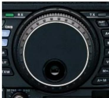
The Main Tuning Dial is a new dual structure, utilizing the normal dial structure along with a rotating skirt that creates a small air gap. This air gap reduces sweat accumulation on the operator's fingertips, enhancing tuning precision during long operating sessions, especially on DX-peditions to hot tropical areas.
