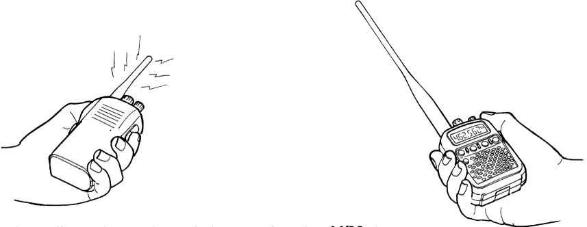
1. Set the radio to the VFO mode by pressing the [V/M] key.
