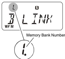
*Now again press and hold in the [FUNC] key, and rotate the **DIAL** knob to select other Memory Banks to be included in (or excluded from) the Preferential Bank Scanning List. Release the [FUNC] key, and rotate the **DIAL** knob to apply or remove the "." from the selected Memory Bank. Press the [SCAN] key while pressing the [FUNC] key when all Bank selections have been made.*
